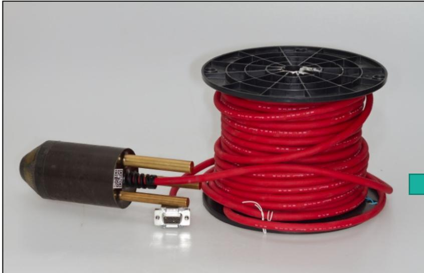
CCBM (Compact Conical Borehole Monitoring) probe installation with same principles as CCBO probe without overcoring process
